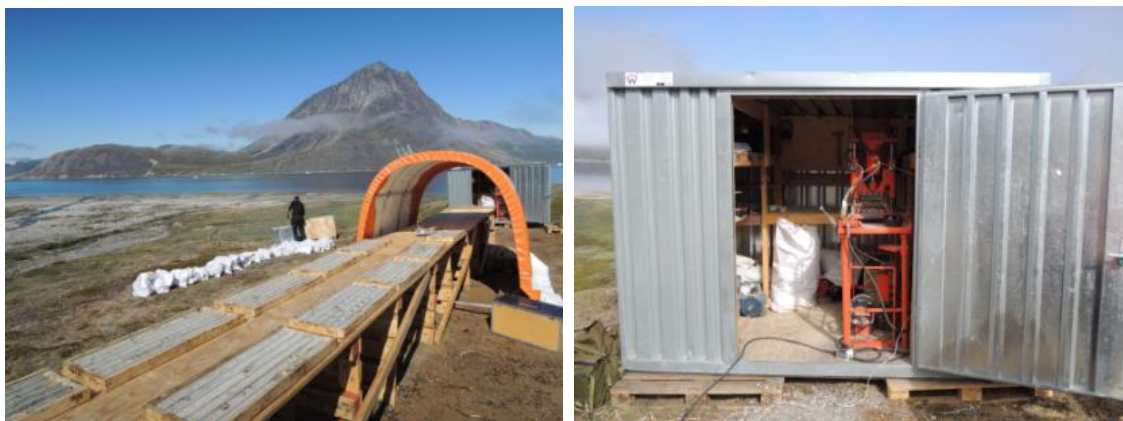
Figure 11-1: Core logging table and temporary sample storage at the Qoorormiut delta (left photo). Core cutting shed and hydraulic splitter (right photo) (SRK, 2012).
